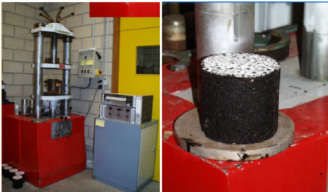
Figure 3: PCG apparatus (left) and test sample (right) [Source: 3 E's 4 Africa e.V., 2022]
