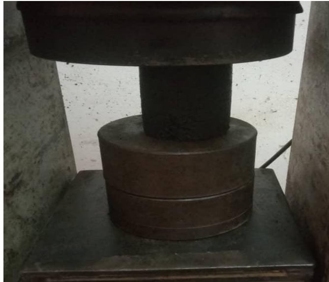
Figure 1: Crushing of a Duriez test specimen [Source: 3 E's 4 Africa e.V., 2022]
