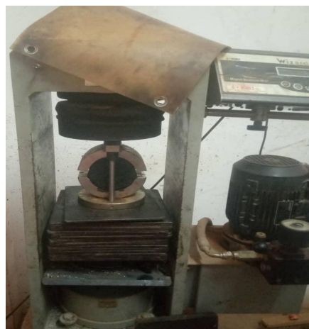
Figure 2: Crushing of a Marshall test piece [Source: 3 E's 4 Africa e.V., 2022]
